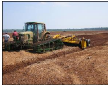
Figure 1b – Crowning the fields with a screw leveller
