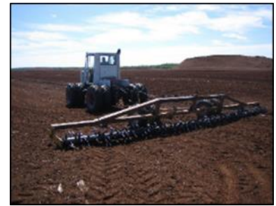
Figure 1c – Harrowing the surface to loosen and fluff the peat moss
