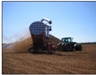
Figure 1e – Dumping the collected peat at the end of the production fields
