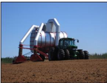
Figure 1d – Collecting the dry surface peat layer with a vacuum harvester
